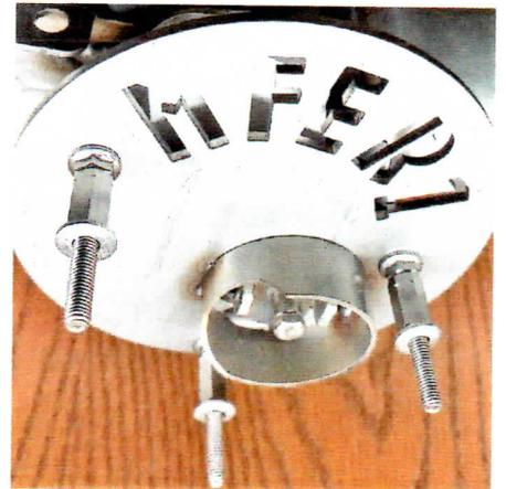
Next install 3 small flat washers, then 3 serrated washers with lines facing out.
