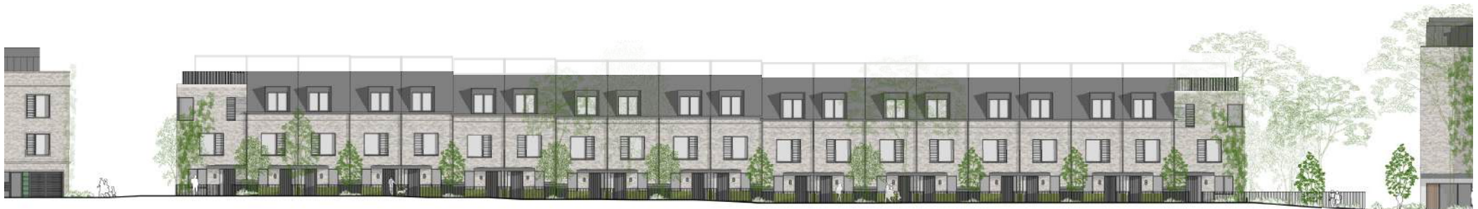
Proposed Block B north elevation showing lower masonry to align with 7 Collins Street, dormer windows, book-end units, and front gardens
