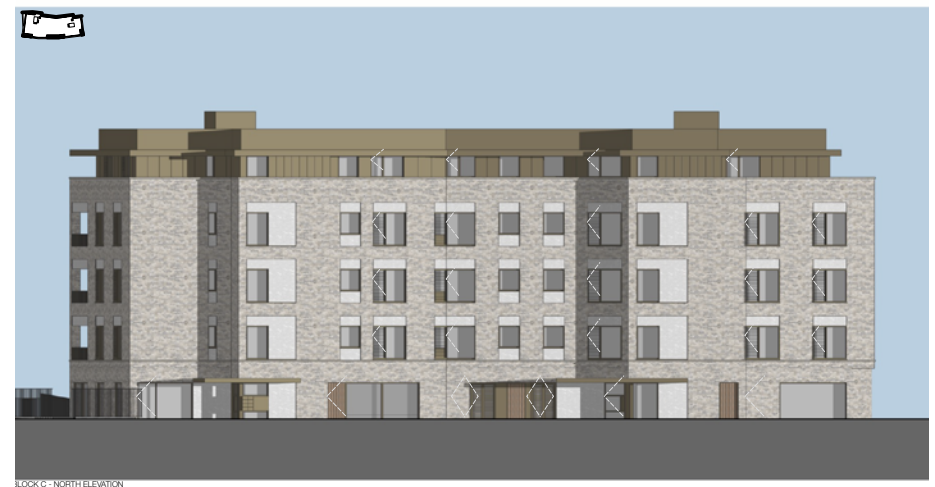
Elevation studies by JPA after DRP 02 exploring a formal elevation treatment to Block C akin to Mansion Block typology studies. Proposal deemed problematic owing to reduction in opening to recessed balconies
