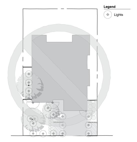
Avoid excessive lighting, "runway" effects and unbalanced configurations
