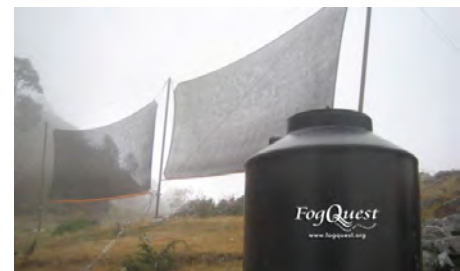
"Atrapanieblas" fog collection in Alto Patache, Atacama Desert, Chile
