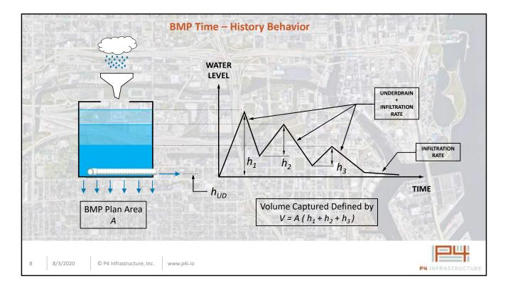
This schematic is the behavior of a permeable pavement storage reservoir over time.
