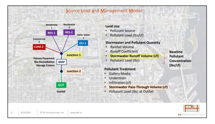
After the no-controls analysis, proposed stormwater best management practices (BMPs) are added to the model.
