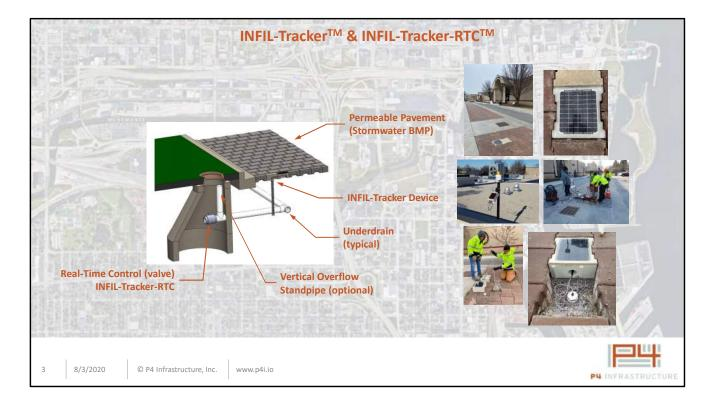
To answer these questions, P4 developed INFIL-Tracker and INFIL-Tracker-RTC to monitor in-situ performance of permeable pavement systems.
