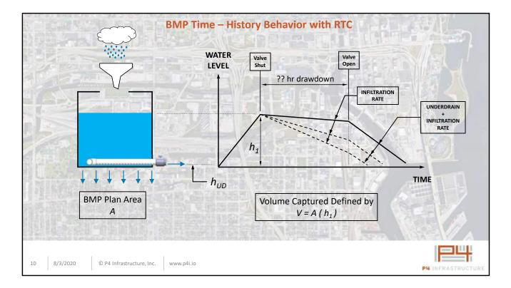
This is the behavior of the BMP with real-time control (RTC) added.
