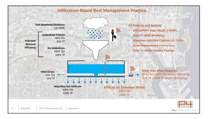
Here's a side-by-side scenario schematically showing a permeable pavement BMP with and without INFIL-Tracker-RTC.
