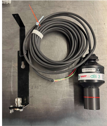
UT Sensor with Manhole Mounting Bracket
