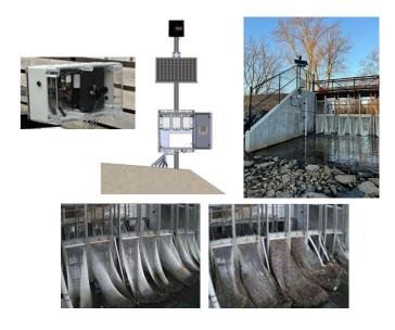
CamVIEW is a robust autonomous image capture system for stormwater trash collection infrastructure.
