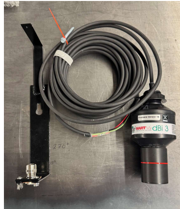
Pulsar Measurement dBi UT Sensor with Manhole Mounting Bracket
