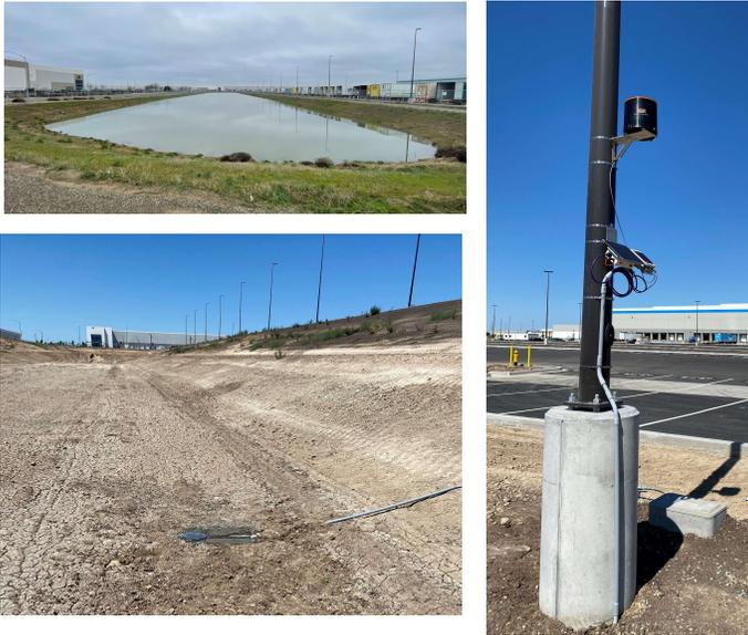
LIQUA-Level EPC is a robust water-level and sediment measurement system for stormwater infrastructure.
