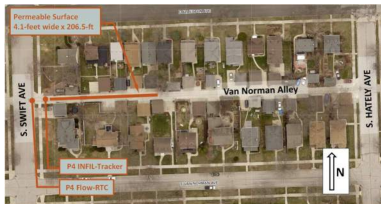
Figure 1. Van Norman Alley permeable pavement installation with monitoring system locations.
