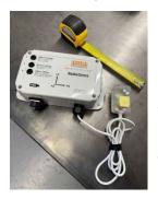
makes it suitable for outdoor use. It 120V uses reliable power. ShakeSense-2<sup>™</sup> is а selfcontained, portable device with no maintenance required. The sensor. computer, and electronics come together in one physical unit to form an all-in-one solution. ShakeSense-2<sup>™</sup> is a stand-alone, maintenancefree, short-term vibration monitoring solution.
