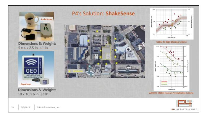
P4's solution for vibration monitoring is called ShakeSense. ShakeSense is a low-cost, small form factor, vibration monitoring system for evaluation of structural damage, nonstructural damage, and human perception of vibrations.
