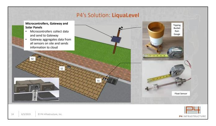
P4's solution to aid in stormwater management is LiquaLevel.
