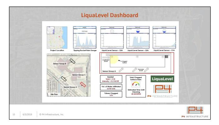
This is one way that users can interface with the data collected by LiquaLevel sensors. Permeable Pavement owners can view the data from each sensor and gain a better understanding of how their system is functioning throughout the service life of the asset. For example, they can get vital information like: When do I need to clean my pavement?
