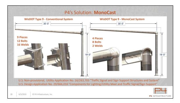
P4's patent-pending solution is called MonoCast: Monotube structures utilizing steel castings.
