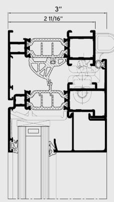
Concept System® 77 is a high-insulation window and door system that meets elevated requirements regarding thermal insulation, stability, and security. CS 77 is available in a variety of aesthetic styles to match the current trends while offering all types of inward and outward opening windows and doors. An additional asset is the possibility to combine this system with Ventalis®. The system's performance regarding acoustics, water-, and air-tightness meets the highest of standards.
