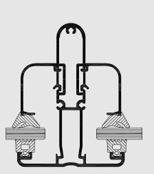
PR 100 is a non-insulated aluminium roof system that can be used as a terrace covering or a carport. PR 100 offers a range of rafters in different heights and widths so that high static requirements coming from snow load and own weight can be implemented without using steel reinforcements.
