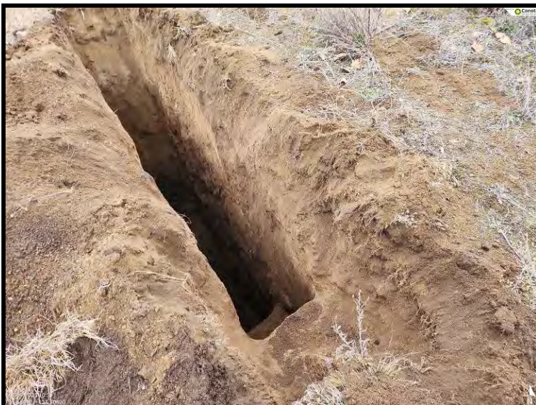
Exposed subsurface soil profile within test-pit TP-5
