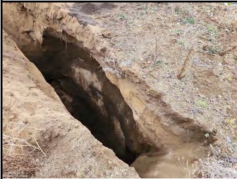
Exposed subsurface soil profile within test-pit TP-1
