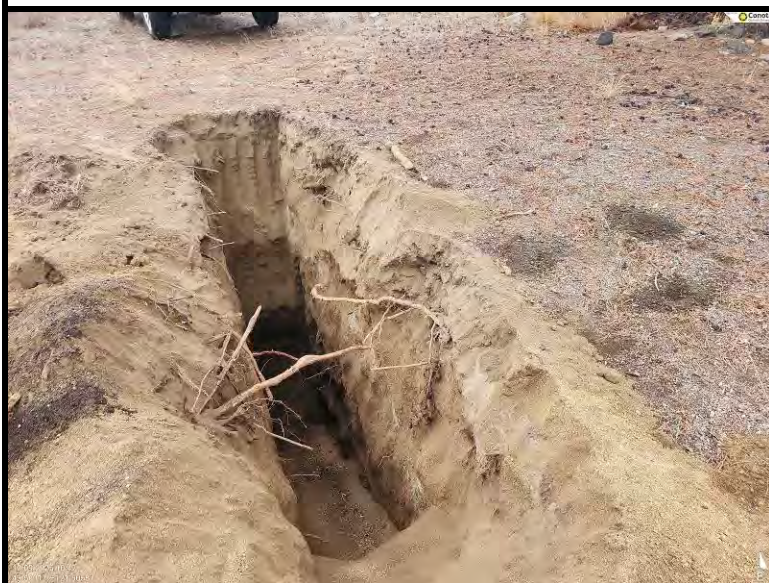
Exposed subsurface soil profile within test-pit TP-6
