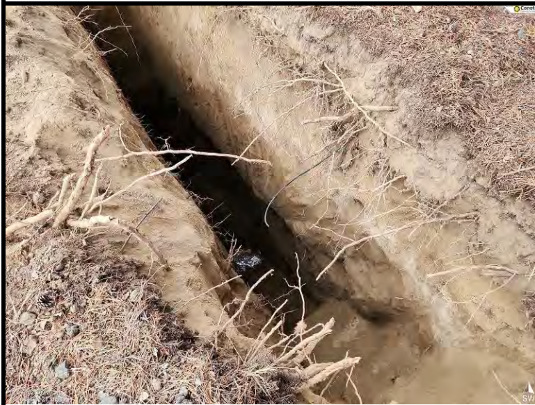
Exposed subsurface soil profile within test-pit TP-2
