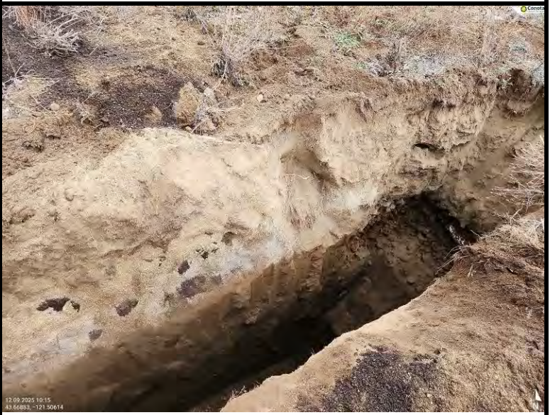
Exposed subsurface soil profile within test-pit TP-4
