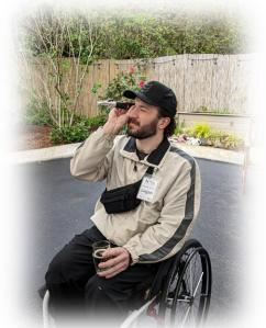
Checking the Specific Gravity (SG) using a refractometer
