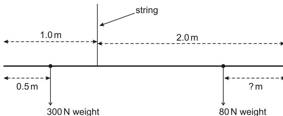
How far from the other end must a weight of 80N be placed for the beam to be balanced?
