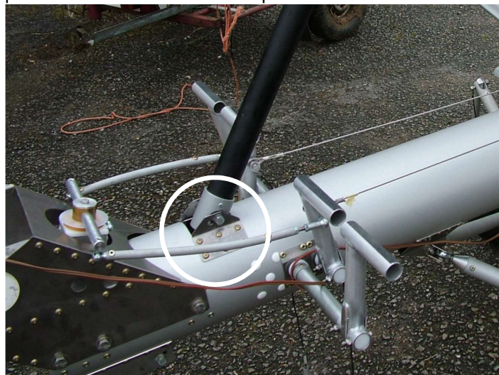
Figure 1: A- pillar attachment to upper surface of main fuselage tube. Lower attachment bolt visible beneath main fuselage tube at aft end of bracket attached to nose leg.
