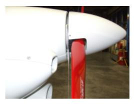
Tie down point between the engine cowling and propeller spinner.
