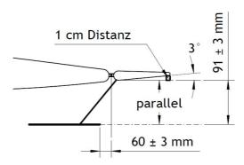
Measurement with water level at base of 1 cm under Aileron end strip.
