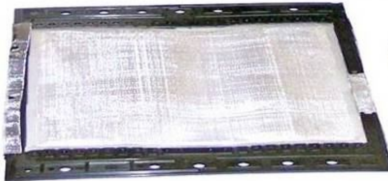
NICKEL SCREEN SURROUNDED BY PLASTIC FRAME FOR LARGE ELECTRODE
