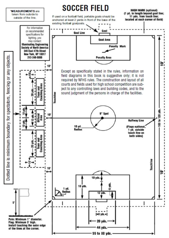
An engineered natural turf soccer field should have a minimum of one-and-one-half percent (1.5%) slope for fields which are surface drained. For natural turf fields with a sub-surface drain system the slope should be no less than one (1.0%) percent. For synthetic turf fields with a sub-surface drain system the slope should be no less than one half of one (0.5%) percent. Slope is measured from center to side. For consulting services, contact SportsPLAN Studio, 816-842-5200.
