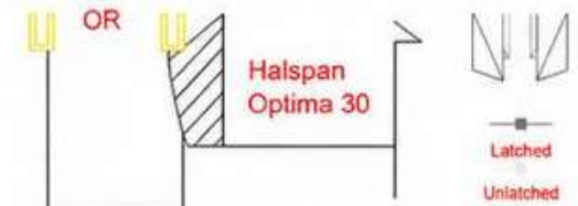
Jamb: All door widths - 10x4 seal
