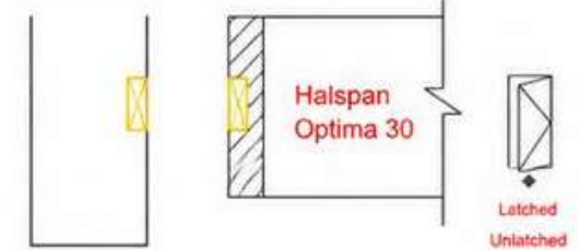
Overpanel back-fixed through frame
