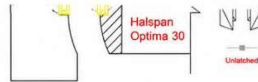
Scalloped Jamb: All door widths - 10x4 seal
