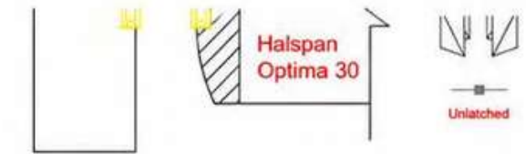
Square Jamb: All door widths - 10x4 seal
