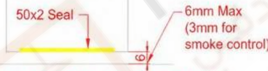
Typical Head / Threshold with R90 seals
