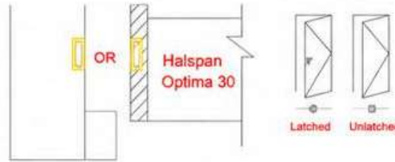
Jamb: Door widths up to 950mm - 10x4 seal
