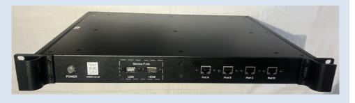
Simulates the RNC / core network and provides all required S1 signalling to the base station
