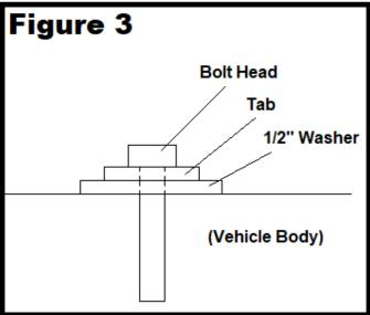
8. Place washers on 1/4" bolts and insert them into the slider mount tabs.
