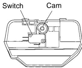
This microswitch is mounted behind the controller at the front end of the camshaft. The switch is mounted to the top plate. The cam for this switch is screwed to the front of the camshaft. This cam can be adjusted to activate the microswitch at any time during the regeneration cycle.
