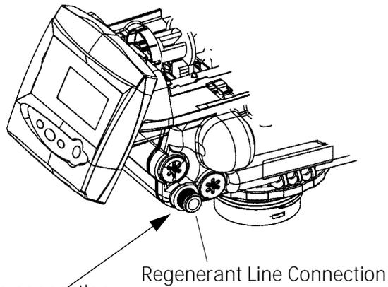
**NOTE:** Be sure to use plumbing connection tube when attaching regenerant line connections to the Performa valve.
