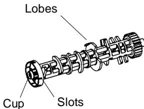
The outside surface of the cup has an arrow mark. When the arrow is at top center, the camshaft is in the loading position. 90 degrees clockwise on the cup an optical sensor is mounted to the top plate. This sensor reads the slots as they pass through. The largest slot is "Home" and the remaining slots are positioned to signal the regeneration cycles.
