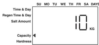
To have your system regenerate on demand, set your system's capacity (P7) to the appropriate factor. On the 760, it will read Kg, but you will actually be working in ppm of iron.
