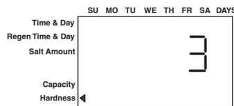
1. If your system is one cubic foot, set the capacity to "10" kg, meaning 10,000. For two cubic feet, set the capacity to "20" kg.
