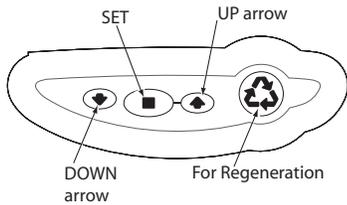
The 700 Series controllers are designed to operate by only setting the time of day and the day of the week. The remaining settings have been set at the factory. These default settings will work for most applications.
