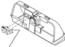
Do not bend the legs on the optical sensor
