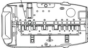
Inspect valve discs for wear. The sealing surface is the raised ridge on the underside of the top shoulder.
