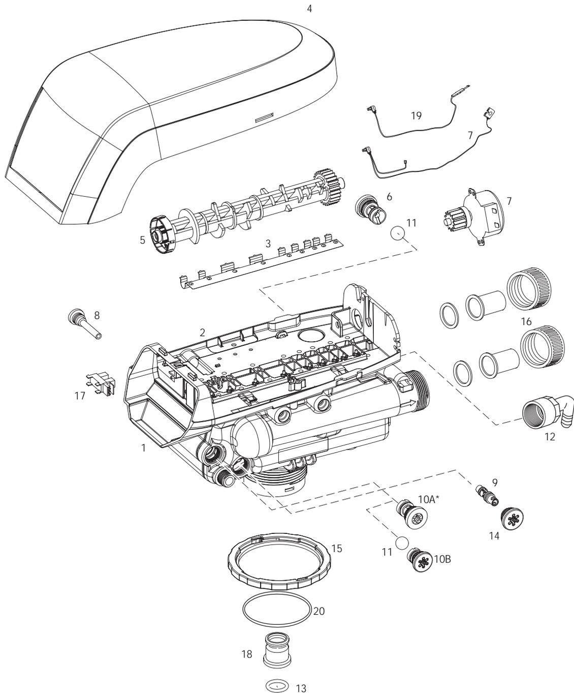
\*Warning: Do not use the flow control ball with #10A.
