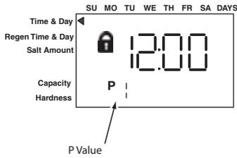
The 740/760 features a special programming level that allows the installing dealer to make changes to the control for more demanding applications. The home owner/end user should never have to access this level.
