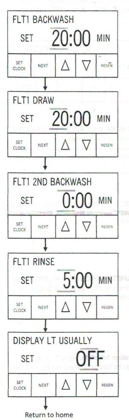
Step 6I-IZ – Select duration of 1st cycle. Use ▲ or ▼ to select value other than default value. Setting will flash when changed from this initial value. Press NEXT to go to Step 7I-IZ. Press REGEN to return to previous step.
