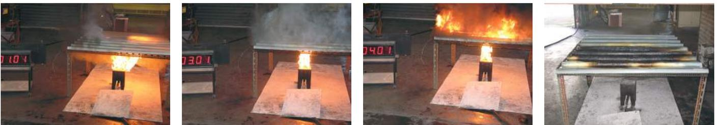
The top surface of the SL Fire Retardant achieved a peak temperature of 652.7°C and was reached at 265 seconds as the sheeting became engulfed in flames.
