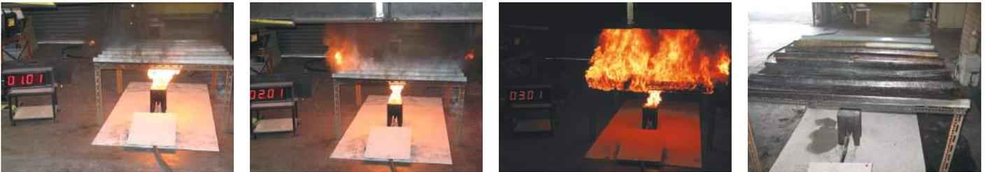
After three minutes, the sheets were doused with water extinguishing the flames. Heavy black smoke was abundant creating a time delay wait for fumes to be exhausted. The result of the fire is evident with the front sheet ready to collapse.
