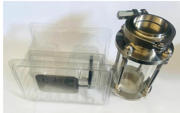
Experiment Tri-Clover Sight Glass, Mounting Flange and BS&B Rupture Disc
