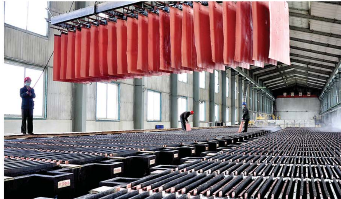
Electrolytic copper production
