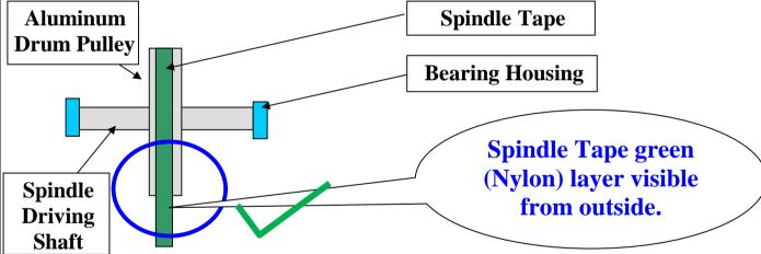
Off white (Cotton) side of Spindle Tape must be in contact with Drum Pulley. Contact of green side (Nylon) will lead to slippage of Spindle Tape. In case of abnormality inform to Maintenance Team
