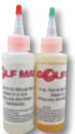
9819 / Long Cure Epoxy 8 oz Kit (two 4 oz bottles) 20 - 30 Minute setup 12 - 20 Hour Cure Full cure lap shear strength 3450 psi
