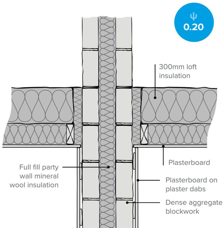
Use lightweight aggregate blockwork for the party wall leaves to improve thermal performance.
