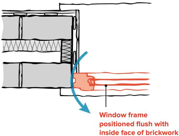
Window frame positioned flush with inside face of brickwork
