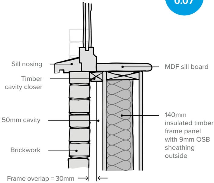
Use a cavity closer with a PU/PIR insulation core to improve performance of sills and jambs.
