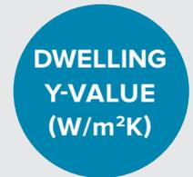
The sum of the individual junction heat losses divided by the total exposed surface area of the dwelling gives the **Y-value**. The Y-value expresses the overall heat loss arising from all of the building junctions as an equivalent U-value for the dwelling.
