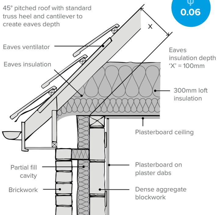
**Use insulated plasterboard on inner blockwork leaf to improve eaves performance.**
