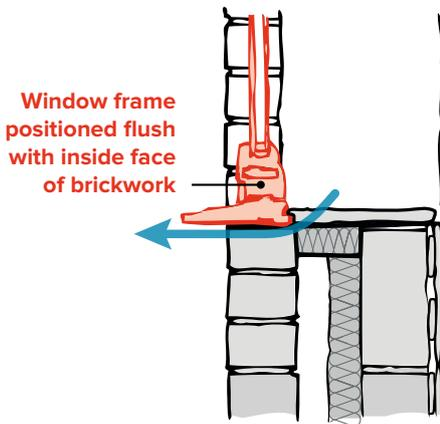
Window frame positioned flush with inside face of brickwork
