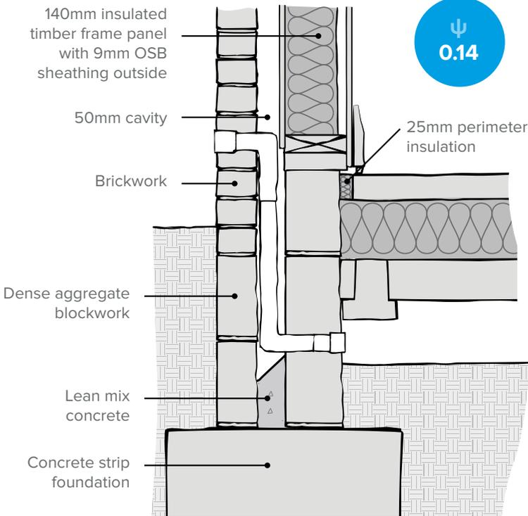
Increase the perimeter insulation thickness to improve ground floor performance.
