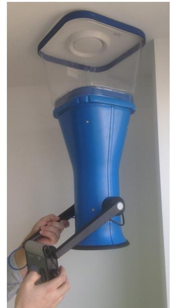
MEASURE AIRFLOW WITH APPROPRIATE DEVICE
