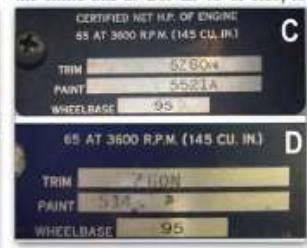
1963 Rampside cowl plates (C) from Saint Louis with prepended "S" and (D) from Flint lacking "S" and paint code ECL. (E) Cowl plate from 1964 Greenbrier with new two-
