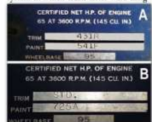
Figure 1. (A) 1962 Greenbrier cowl plate from Saint Louis with Custom Equipment Trim code. (B) 1961 Rampside cowl plate from Saint Louis with "STD" Trim code.
