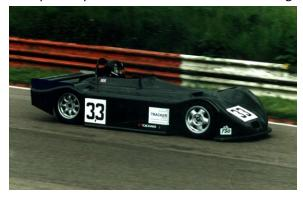
was desperate to try it so I modified the existing mould and did a wet lay-up carbon body, this time in three parts to aid component access.
