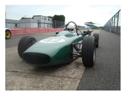
I took what I think is an unusual approach in designing the Falcon in that I have given much more consideration to the driver as part of the system making sure that the ergonomics of the brakes and steering optimises feedback and control for the driver and that the basic handling characteristics and transitional behaviour of the car are stable and predictable. If the car is in any way awkward to drive then an amateur driver will not get the best out of it in only 15 minutes of practice.
