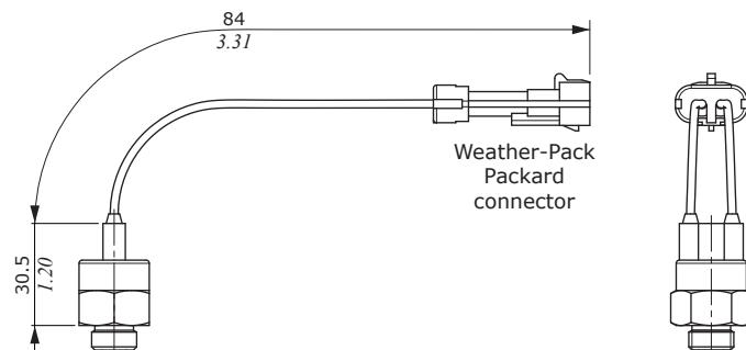
**Example of sensor in 8MG control with SD8 working section**
