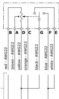
Interface: to use the joystick redundancy option, this wiring is required
