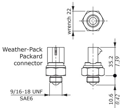
**Sensor with connector and flying leads**
