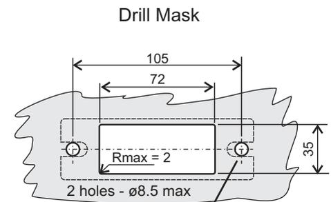
Mounting screws must be sealed apart (rubber gasket does not seal them)
