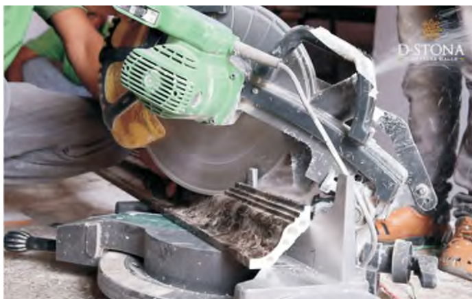
Molding cutting using a miter saw.
