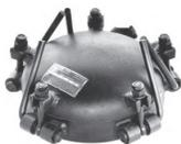
**T-Bolt Closures** are designed for nominal pressure applications. T-Bolt closures are available for horizontal and vertical applications in sizes 6" - 66" for pressures up to 300 psi.
