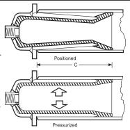
And when the test is finished, the SWEL-PLUG Pressure Tester can be removed with a minimum of effort because its grip to the pipe walls slackens automatically as internal pressure is relieved.
