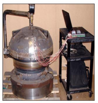
24" CL900V Closure under 3350 psi Hydrostatic Test
