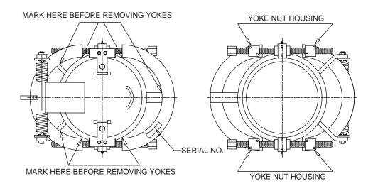
**Disassembly Procedure:** Numbers in () refer to Parts List on following page. Before commencing disassembly, be sure to observe the warning and precaution under Operation.
