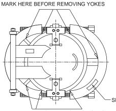
MARK HERE BEFORE REMOVING YOKES **Disassembly Procedure**: Numbers in () refer to Parts List on following page. Before commencing disassembly, be sure to observe the warning and precaution under **Operation**.
