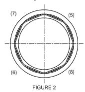
c. Complete the installation by pushing the O-ring into the groove in between the initial installation points above. If the O-rings are of a high hardness (90 durometer) or are being installed in cold weather it may be necessary to use a block of soft wood and a small hammer to tap the o-ring into its fully seated position in the groove.
