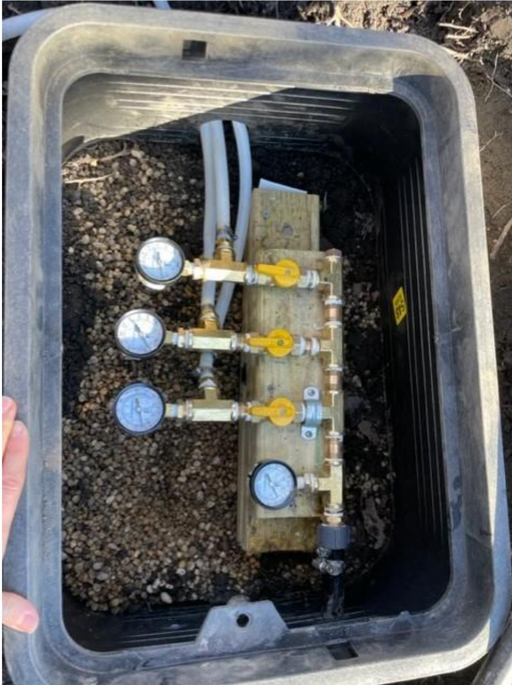
**Figure 4:** Photo of the air injection manifold facilitation air injection to the 3 gravel columns. Manifold includes valves and gauges to allow pressure monitoring and adjustment.
