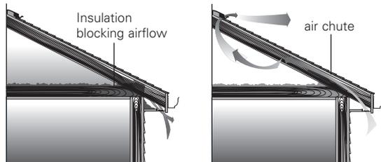
*Figure 7-10: (Left) Insulation should not be installed over the soffit/undereave intake area or proper inflow to the attic will be impeded. (Right) An unblocked vent allows a passage for air to move through the attic.*
