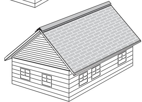
Figure 7-21: (Top) Ridge vent shorter than the ridge length presents an unattractive “broken” appearance. (Bottom) A ridge vent should extend all the way from one end of the roof to the other end of the roof for a smooth “unbroken” roofline.
