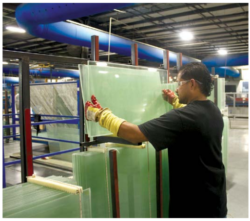
After the glass exits the infrared oven, it is stacked on racks. In the final step of the lamination process, the racks are heated in the autoclave at 270°F, 170 psi for 3.5 hours.
