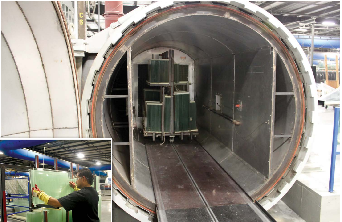
After the glass exits the infrared oven, it is stacked on racks. In the final step of the lamination process, the racks are heated in the autoclave at 270°F, 170 psi for 3.5 hours.
