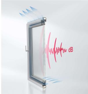
The Schüco AWS 90 AC.SI acoustic window is a single-skin window solution for natural ventilation with simultaneous sound reduction, which can be up to 34 dB depending on the design option. This new window can be used to provide natural ventilation, while keeping noise levels in the building low. Rooms such as bedrooms and children's rooms on the sides facing the street, can be naturally ventilated with this window system, without being disturbed by traffic noise
