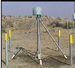
CORS Base Station providing published coordinates
