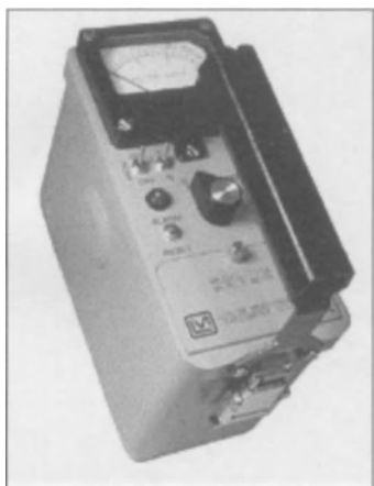
Figure 7.12 This radiation detector is used to detect levels of radioactive materials.
