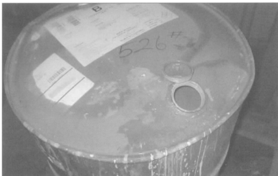
Figure 11.16 A bulging drum is found at a waste site. Opening the drum was done very carefully, so as not to spill contents or expose the entry team.
