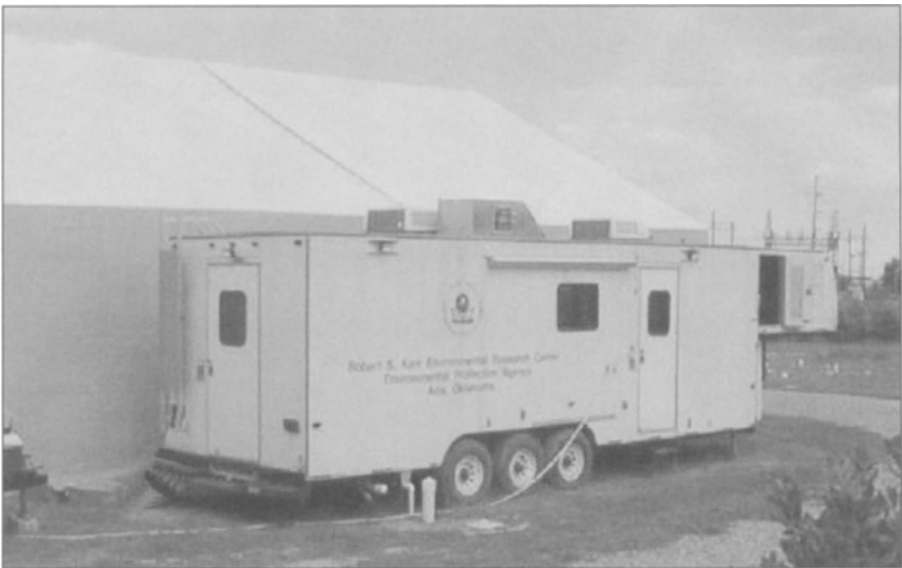
Figure 7.14 The EPA often uses their mobile lab (shown above) for field testing. Mobile labs give faster results than sending samples to fixed labs.
