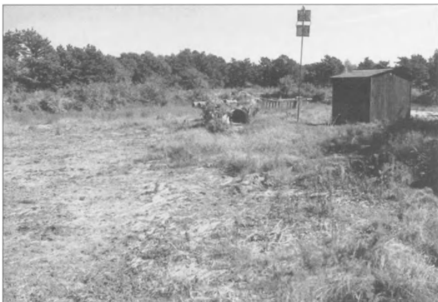
Figure 4.9 Sampling was taken from this area in Massachusetts due to ground water contamination. Note the change in vegetation and discolored soil.
