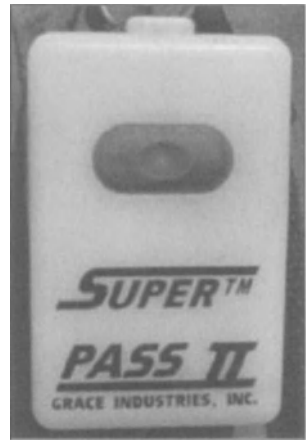
Figure 12.2 This special alarm worn on the firefighter's bunker gear or worker's PPE is activated by the wearer as soon as he arrives at the fire scene/site. The P.A.S.S. alarm contains a motion detector. Should the firefighter/worker become trapped or overcome and remain motionless for a short period of time the P.A.S.S. alarm goes off making a loud noise for other workers in the area to hear and come to his/her rescue. The P.A.S.S. alarm can also be manually set off by the wearer if he/she gets in trouble.
