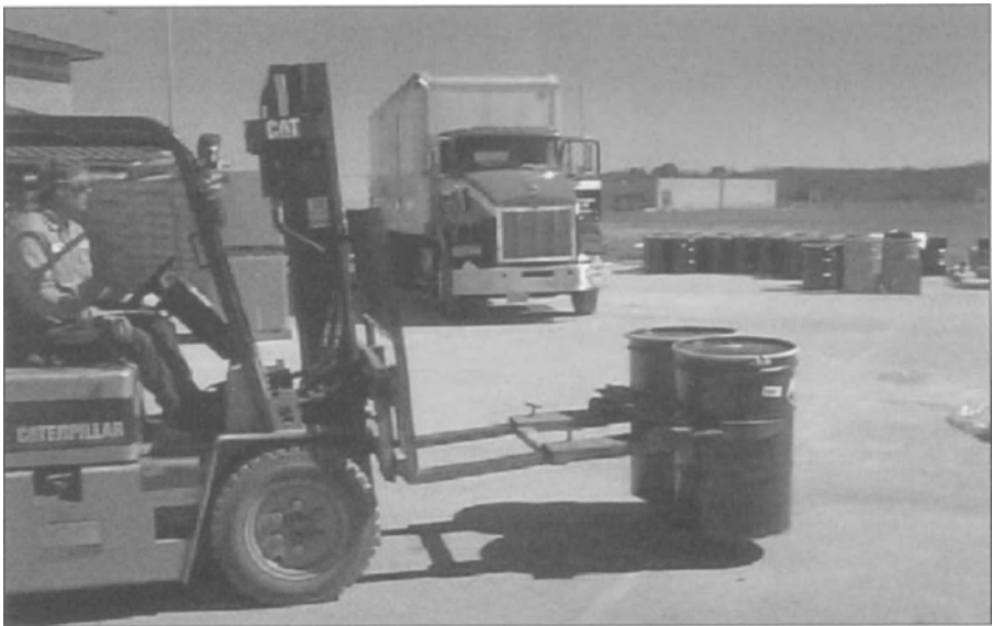
Figure 11.18 A drum grapple moves two drums safely.
