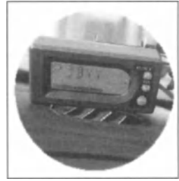
Figure 5.15 This unit allows supervisors to track a piece of heavy equipment if stolen.
