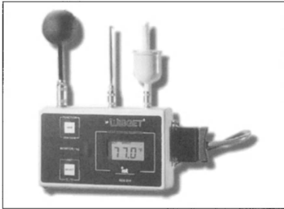
Figure 8.17 A wet bulb globe thermometer is used for heat evaluation.
