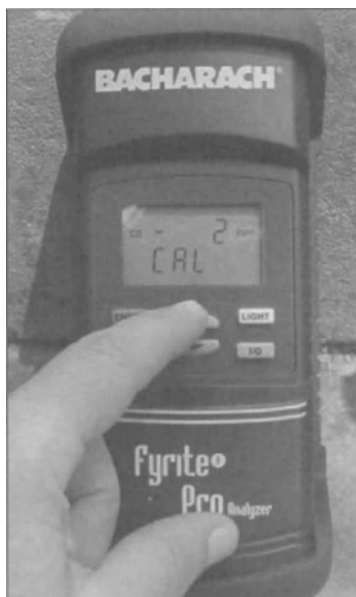
Figure 7.7 Here an instrument is being calibrated in the field.
