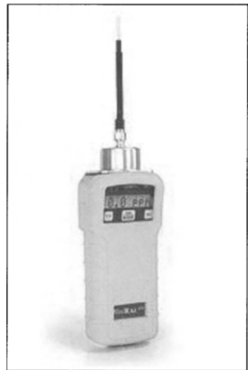
Figure 7.11 This Photo Ionization Detector can be used by workers in emergencies or at waste sites.
