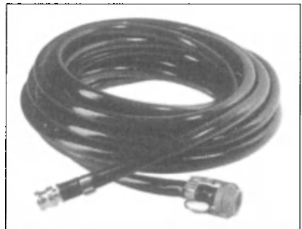
Figure 10.10 Airline respirator hose is shown above. The airline hose is restricted to no more than three hundred feet by OSHA.
