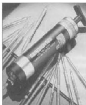
Figure 7.5 A Sensidyne pump is shown above. The air is drawn through the pump by pulling the handle back.
