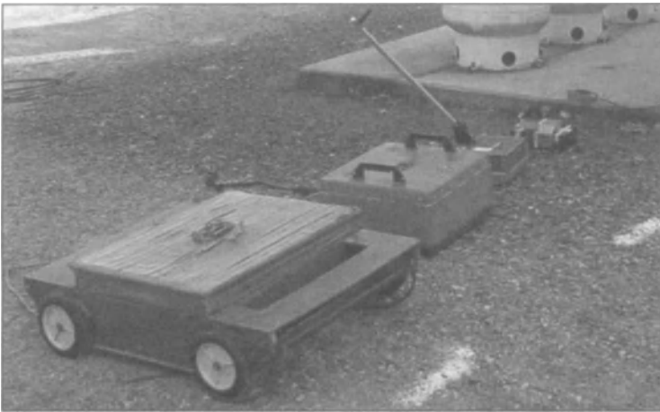
Figure 4.12 Ground penetrating radar is used to detect the presence of buried tanks and drums.
